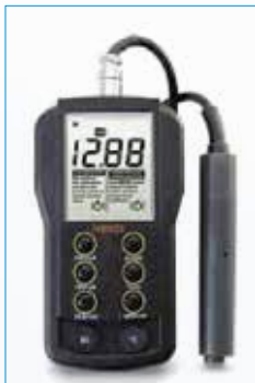
Measurement device for measuring conductivity, pH values and the temperature of the fountain solution
